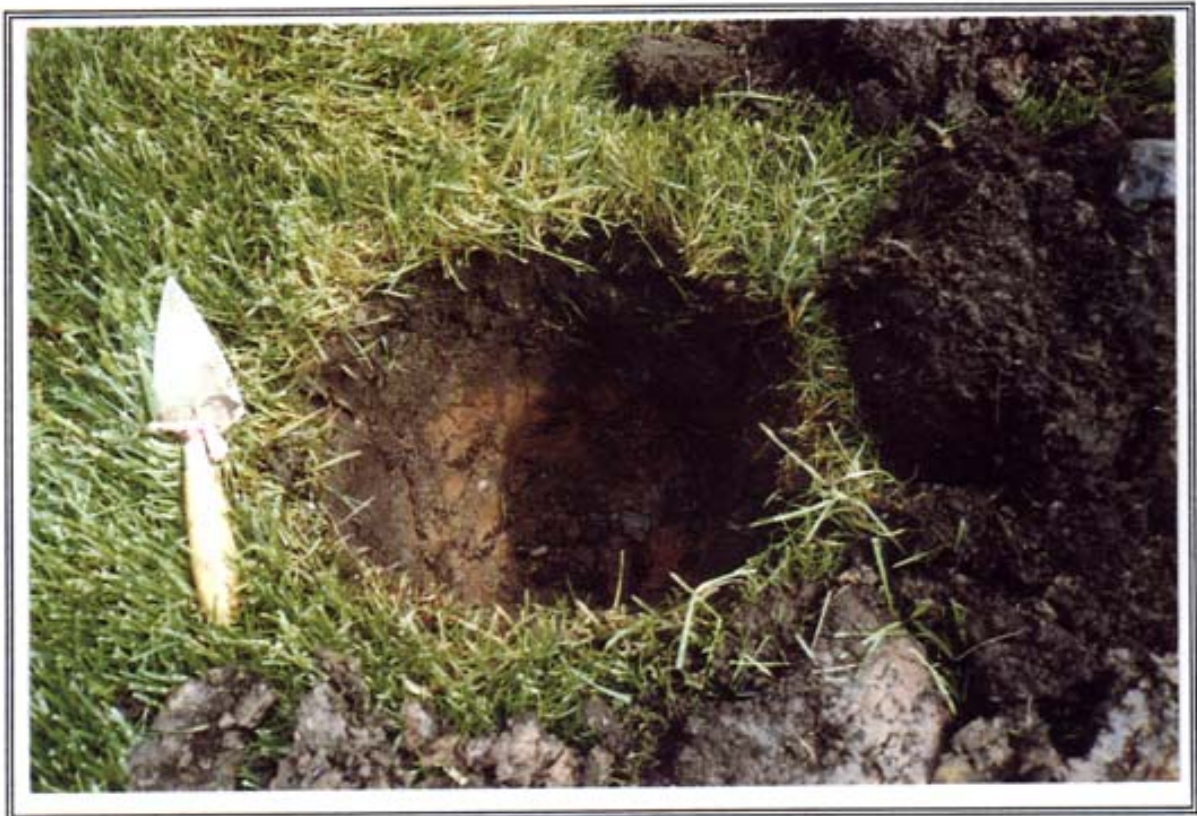
PHOTO 21. 240 VULCAN STREET: Area A - View of Shovel Test Stratigraphy Showing High Degree of Filling and Native Clay Soils.
